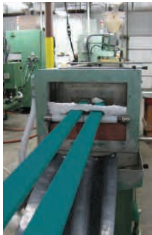
Raw Poly Lumber Exiting Extruder
