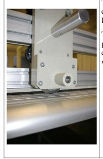
The cutting tool is a very low friction device running on a bearing mounted carriage. The blade has a guillotine action that can cut one or two layers of fabric leaving a quality edge.
