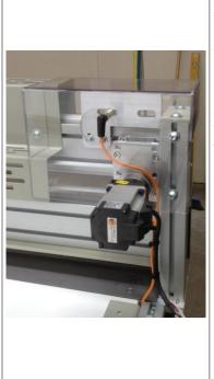
The cutter and/or creaser can optionally be powered so the operator presses a button to drive the cutter or creaser either way.
