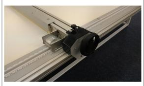
The backstop is full table width, belt equalized, and glides freely. It has a lock down to hold position. A spring loaded stop ensures fabric can't slide under the backstop. The task of the backstop is to make a parallel line to the cut or crease and a right angle to the fabric side guide. This ensures that the final cut or crease dimension is accurate and square.
