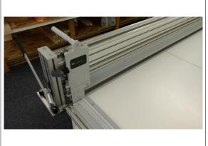
Like the cutting tool, the creasing tool is a very low friction device running on a bearing mounted carriage. The creasing tool is a blunt edge roller instead of a cutter. The blunt edge roller presses the fabric into a groove on the table bed resulting in a sharp, straight crease.
