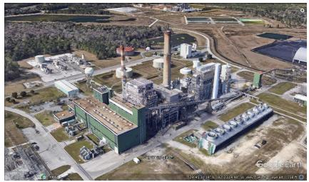
(coal, oil, NG and nuclear). SC-STG's typically have relatively long start-up times (8-24 hours) and are usually restricted in the number of starts and minimum run-time to reduce thermal fatigue and wear on large expensive components.
