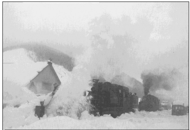
Rotary snow plow, pushed by two "Shay" locis, making a second pass by the Cookhouse.
