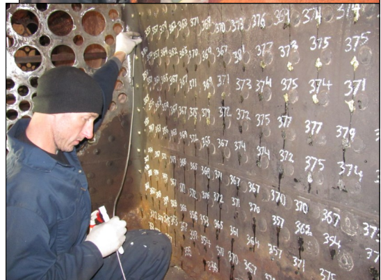
(right, upper) Ultrasound technician scans the boiler shell.
