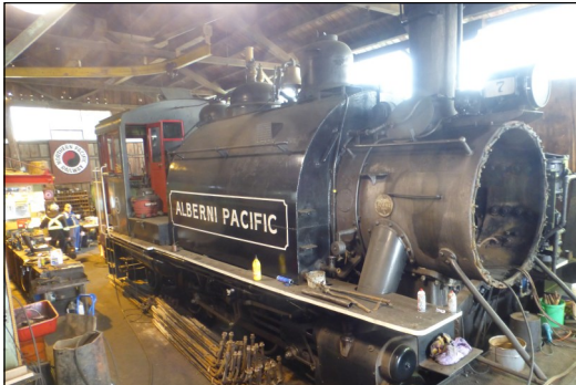
"No. 7" with smoke box cover removed to give access to one end of the boiler, to remove the 134 tubes and 21 superheater flues.
