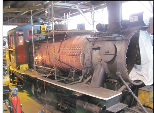
Boiler shell stripped, ready for ultrasound testing The saddle tank and cladding have been removed.
