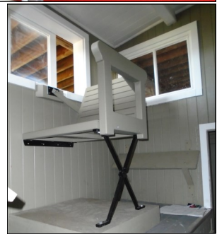
Seat in Cupola the Conductor can view the whole train from up there. There is a seat on each side of the cupola and the back folds.
