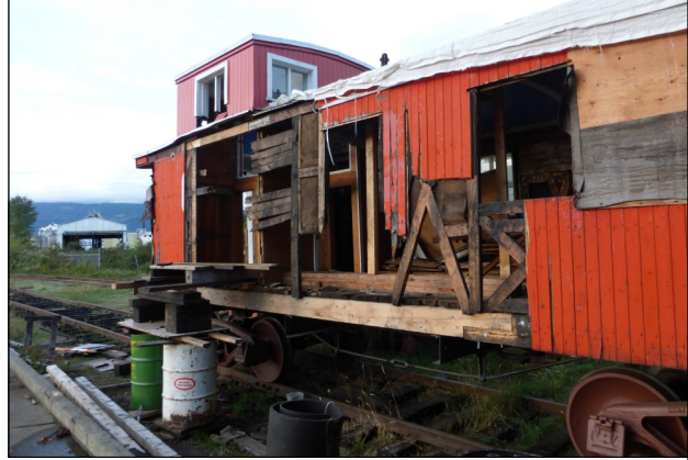
2016 Frank Holm—stripping the other side. (Below) 2014 Stripping rotten framework & siding.
