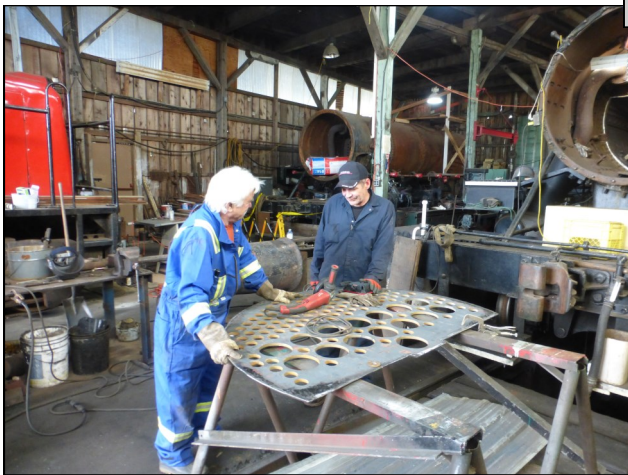
(above) Grinding the surface of the Tube Sheets. Michael Roxburgh & Barry Dobrensky. (Below) Jim Isenor (“Kodiak NDT”) inspects the progress with Michael Roxburgh.
