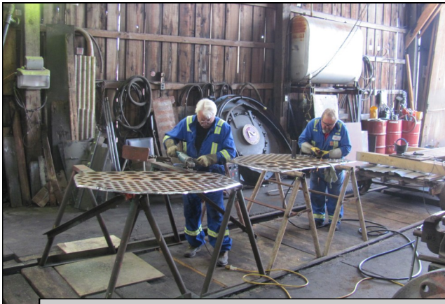
(above) Grinding the surface of the Tube Sheets. Michael Roxburgh & Barry Dobrensky. (Below) Jim Isenor (“Kodiak NDT”) inspects the progress with Michael Roxburgh.
