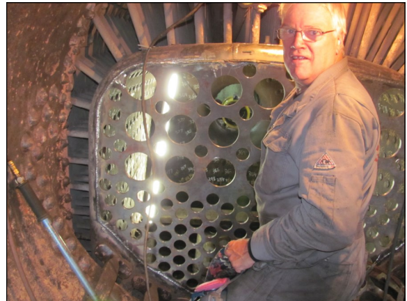
(above) Wrestling a Tube Sheet into the Boiler (left) Rocky checks the fit of the Tube Sheet. (Below) Brent Graham prepares to weld another pass on the Tube Sheet next to the Fire Box.
