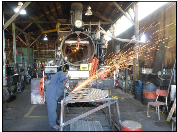
(above) “Bender” at work. Bevelling the edge of the Tube Sheet.
