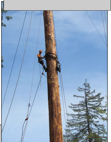
"Meat in the hook" Aaron Thom, High Rigger, is being hoisted up the Spar at the Mclean Mill, on the 'pass line.'
