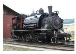
weight and traction as the locomotive's main purpose was for pulling logging trains on steep grades. The engine has a tractive force of 29,100 lbs., burns oil and can carry up to 1800 gallons of water.
