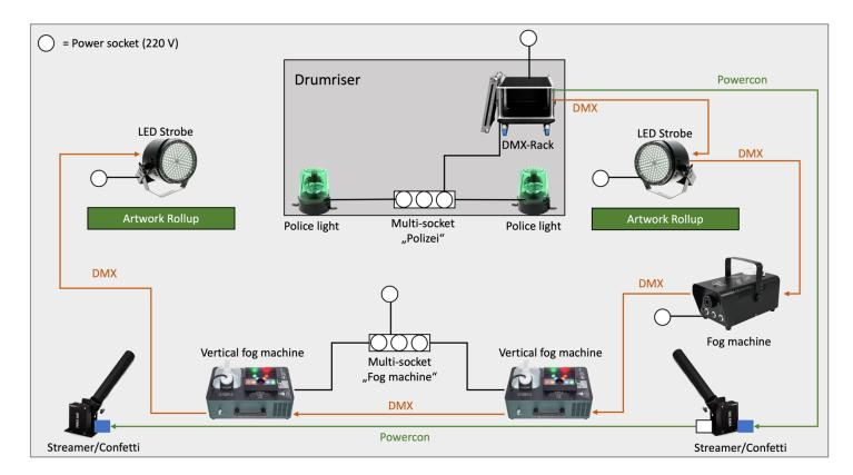
The above plan shows the usual set-up with the necessary cabling. A total of 5 power sockets are required at different points on the stage (DMX rack, 2 x LED strobe, fog machine, vertical fog machines). The multi-plugs in the plan and the remaining cabling will be provided by the band.
