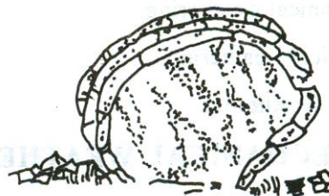
Fig 2.4 Peeling of Layer of the Rock
