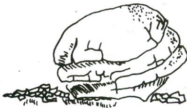
Fig 2.4 Peeling of Layer of the Rock
