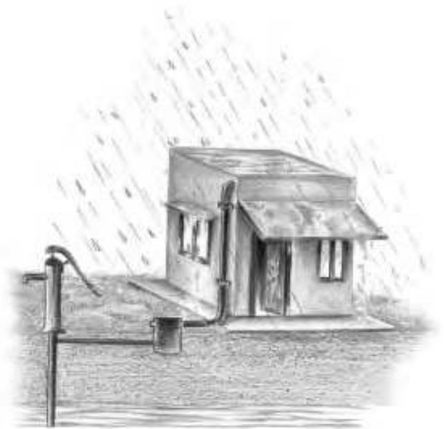
(a) Recharge through Hand Pump
