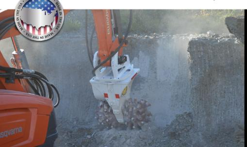
Recommended Excavator/Carrier Size Class: 2 - 8 tons
