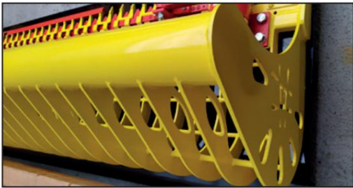
Profile designed for the passage and protection of hydraulic pipes. Profile planned for the passage and the protection of the hydraulic hoses. Profile designed for the passage and protection of hydraulic hoses. Profile for passage and protection of hydraulic hoses.
