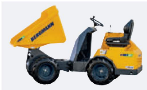
C801e - the little brother with a width of 980 mm and a payload of 950 kg
