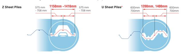
F401 is designed to Press-in a pair of 600mm and 700mm U sheet piles in pairs by using WU chuck attachment.
