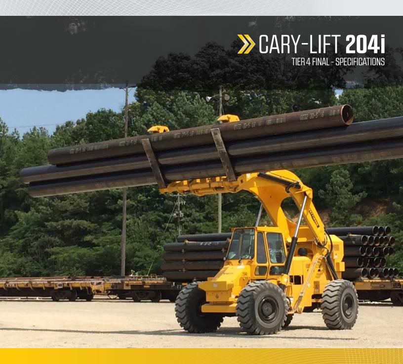
Designed to provide full frontal visibility, the Pettibone® Cary-Lift™ 204i allows operators to lift, place and transport loads with maximum efficiency and safety. A heavy-duty solid steel frame keeps loads stable in full turns. Offering joystick controls and other features for intuitive operation, the 204i provides 90-degree fork tilt down, forward reach, sway control and side shift for unmatched load manipulation.
