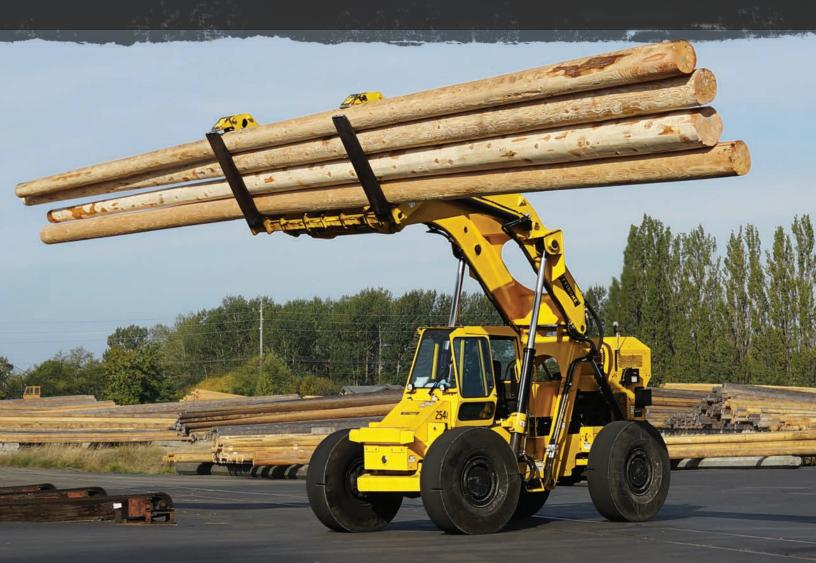
The Pettibone® Cary-Lift™ 254i features an overhead lift arm design that offers full frontal visibility for optimal load handling safety and efficiency. Featuring a load sensing hydraulic system, 225-horsepower engine and heavy-duty 4-wheel drive axles, the 254i is built to take on the toughest material handling jobs, from pipeyard loading to rough terrain applications.
