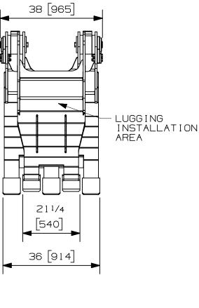
\*\*JAW OPENING WILL VARY UP TO 10% OF SPECIFIC OPENING, DEPENDING UPON THE MODEL EXCAVATOR IT IS MOUNTED TO.
