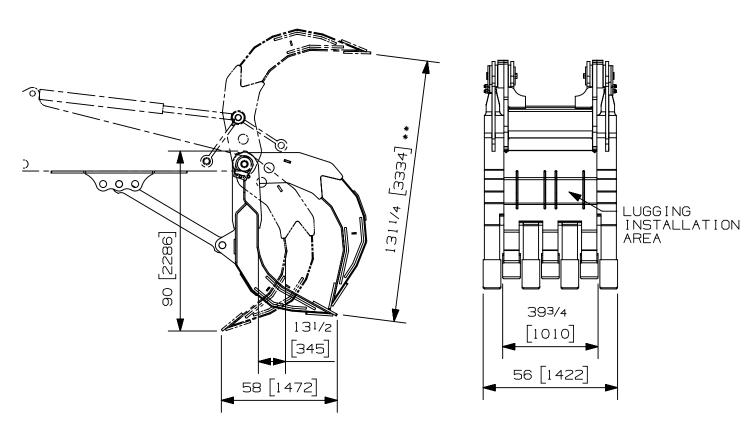
\*\*JAW OPENING WILL VARY UP TO 10% OF SPECIFIC OPENING, DEPENDING UPON THE MODEL EXCAVATOR IT IS MOUNTED TO.
