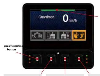
Solid green: Guardman emergency brake System start-up Display switchin button
