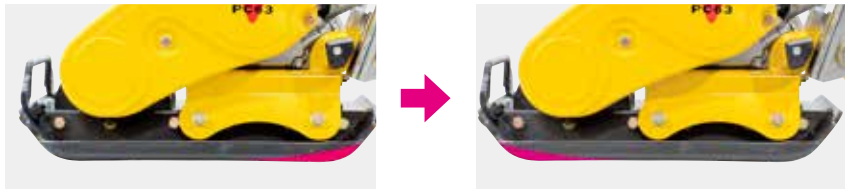
Compaction plate can be turned 180 degrees to prolong the service life.
