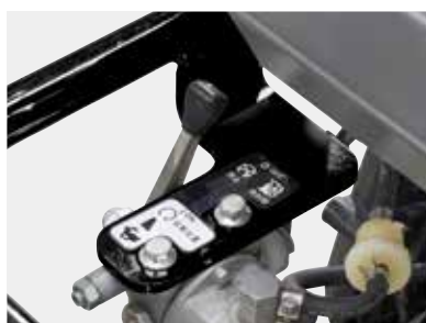
One throttle lever (Engine-off, Fuel-off, Throttle adjustment)
