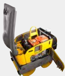
One-touch open covers for easy maintenance
