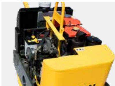
Full-open type cover for easy maintenance
