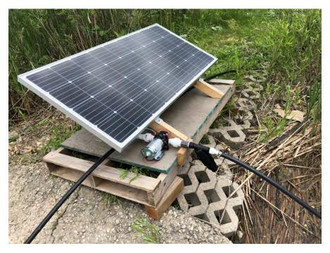
The system consists of a solar panel, a battery and a 12 volt pump which is rated at 3.5 gallons per minute. A timer runs the pump for 40 minutes every day around noon.
