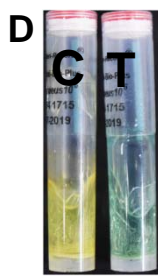
Figure 4. Corncob Disinfection efficacy of OptiMaser at 100°C. (A) Representative plates for total aerobic plate count. (B) OptiMaser parameter at 40min hold time at 100°C and Log reduction in bacteria, spores and Fungi upon OptiMaser treatment. (C) Relation between log reduction and % reduction. (D) Disinfection of 10^6 B. atrophaeus spores upon OptiMaser exposure at 100°C for 30min along with rice husk load. No change in colour of the medium after 48hrs of incubation at 37°C suggest complete disinfection. C, Untreated control; T, Treated vial.
