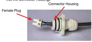
D) Slide Female Plug into the Connector Housing. Be sure to align the keyway on the Female Plug with the keyway on the inside of the Connector Housing. Push all the way down.
