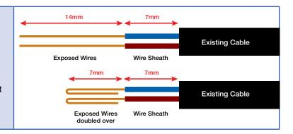
Method B: When using White or Black Cable Seal (thicker cable)
