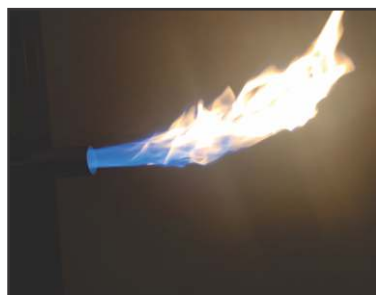
Recommended flame Orange/yellow tip
