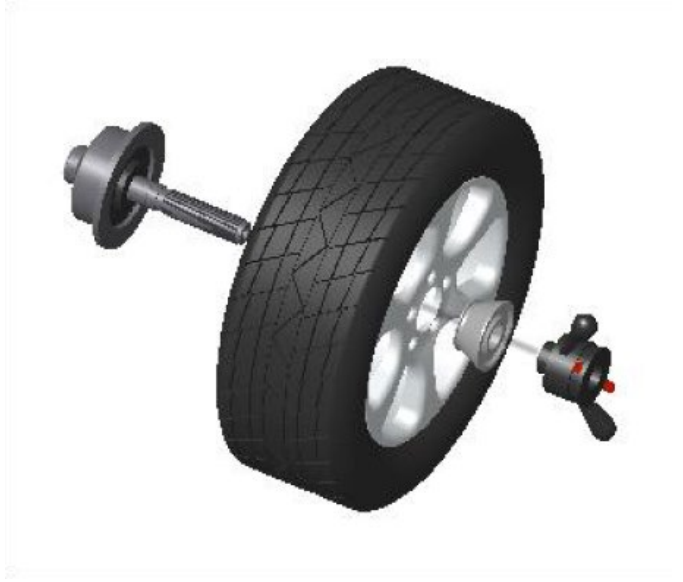
Tensioning on the front
