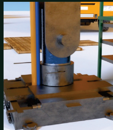
Remove the 2 Chains From the Grooves of the ZSM Coupling to Loosen the Lifting Device
