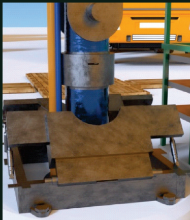
Close both Clamp Doors While the Crane Lower the Pump Unit Until ZSM Collar Seats on the Door Clamps
