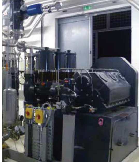
Autoclave feeding, using single-acting FELUWA MULTISAFE® double hose-diaphragm pump in triplex configuration.
