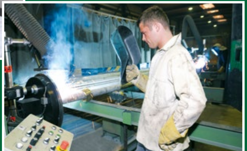
Mechanised welding line
