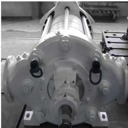
Two flanges in one suction casing
