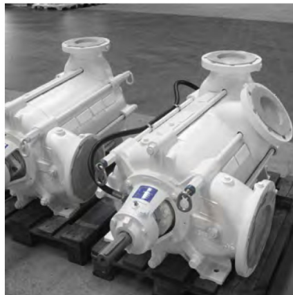
Intermediate flange at stage casing
