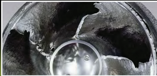
Impeller made of Duplex Stainless Steel Heavy wear after 11,000 operating hours
