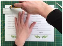
Run your Stanley knife along the edge of the ruler. It's important not to cut all the way to edge of the paper - this way all the crop marks stay intact and can be used for future cuts.
